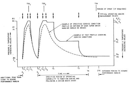
Simulated Service Condition Test Profile
