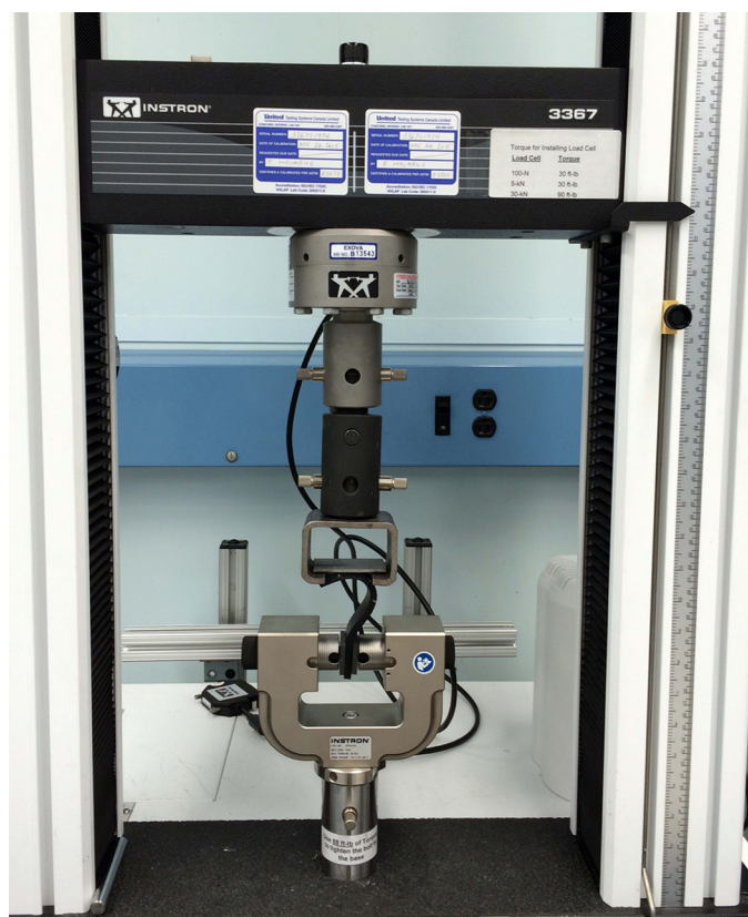
Testing bond strength using an Instron Load Frame in a peeling mode according to ASTM D429 Method B.
