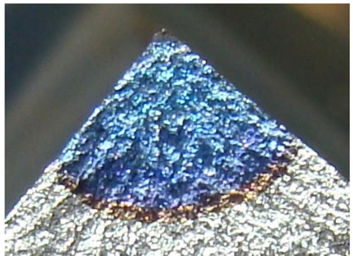
Beachmarks are often observed in fracture faces. They are caused by changes in the load regime or environmental conditions. They are often induced to mark the crack length without damaging the test piece. The images are approximately 10 mm wide.
