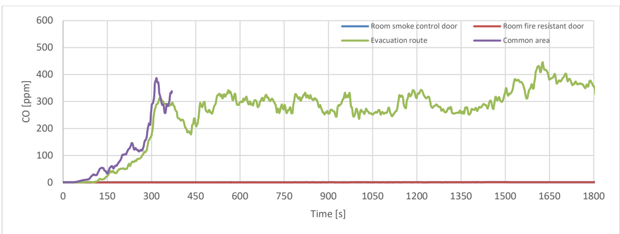
CO content in the rooms and the common area (upper limit measurement: 500 ppm)
