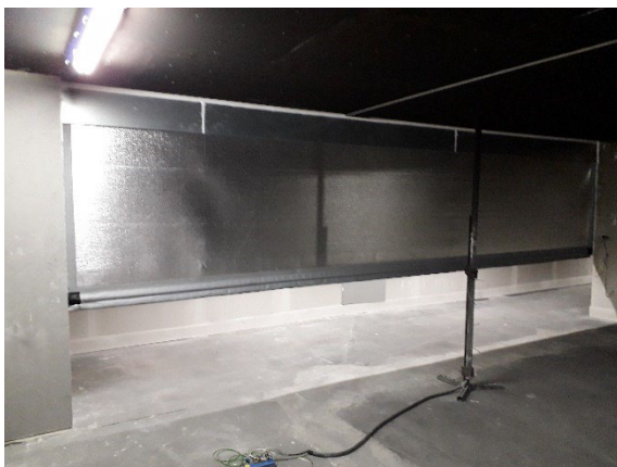
Fire screen up to a height of approx. 0.9 m
